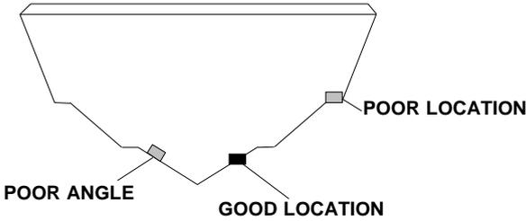
4. Hold the transducer and bracket assembly against the transom. The transducer should be roughly parallel to the ground. The bottom of the transducer bracket should be in line with the bottom of the hull. *Don't let the bracket extend below the hull!* Mark the center of the slots for the mounting holes. Drill two 5/32" holes in the marked locations for the #10 screws supplied with the transducer.
