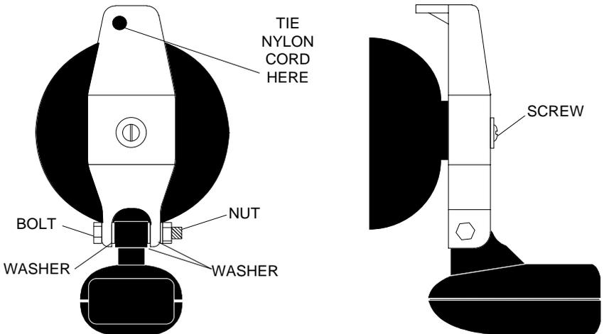
Clean the chosen area of the hull before attaching the suction cup. Locate the transducer on the hull as shown below. Don't allow the bracket to go below the hull, as water pressure against it can cause the suction cup to come off at speed. Moisten the cup, then press it onto the hull as firmly as possible. Tie the nylon cord to the boat and route the transducer cable to the sonar unit. Plug the transducer connector into the unit and your portable sonar is now ready for use.
