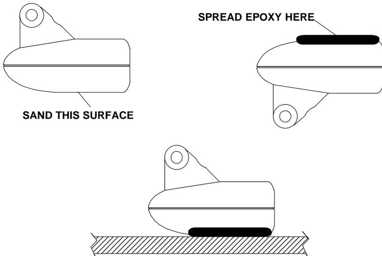
2. Follow the instructions on the epoxy package and mix it thoroughly. Do not mix it too fast, as it will cause bubbles to form in the epoxy. (NOTE! Use only the epoxies specified on the inside front cover of this manual! Failure to use one of these epoxies may result in poor sonar performance!) Apply a small amount on the face of the transducer as shown above, then spread a small amount onto the sanded area on the
