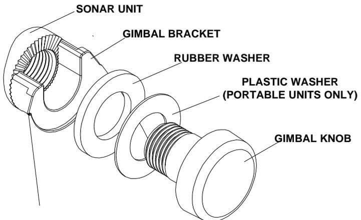
Attach the unit to the gimbal bracket using the supplied gimbal knobs and washers as shown above.
