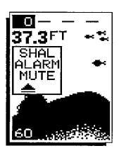
Press the up arrow key to silence the alarm. This will turn the alarm sound off until the shallow alarm is triggered again.
