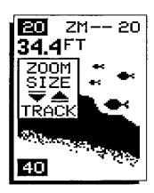
screen. The lower limit is in the bottom left corner. For example, if the upper limit is 40 feet and the lower limit is 70 feet, the zoom window size is 30 feet. The word "TRACK" appears in this menu when you first activate the zoom. This means the Supra J.D. is tracking the bottom in a zoom window, always keeping it on the display.
