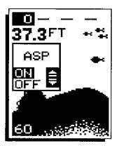
press the up arrow to turn it on or the down arrow to turn it off. The menu will clear automatically after a few seconds or you can press the ON/ CLEAR key to clear the screen.
