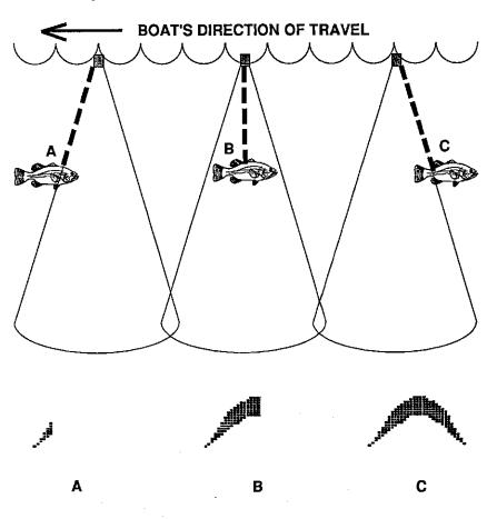
When the Fish I.D. mode is off, the depth of the water will affect the size and shape of the fish arch due to the cone angle diameter. For example, if the cone passes over a fish in shallow water, the signal displayed on the Supra I.D. may not arch at all. This is due to the narrow cone diameter and the resolution limitations of the display.
