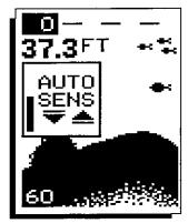
After you've adjusted the unit to the desired sensitivity level, press the ON/CLEAR key to clear the display. If you wait a few seconds, it will automatically clear.
