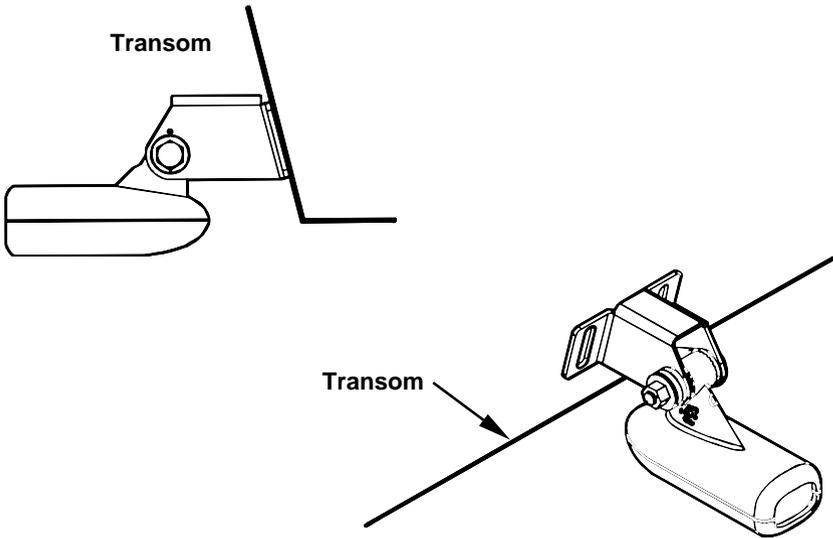
Position transducer mount on transom and mark mounting holes.
