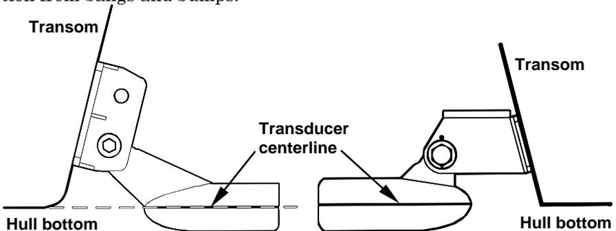
Align transducer centerline with hull bottom. A dual frequency transducer is shown at left and a single frequency transducer at right.
